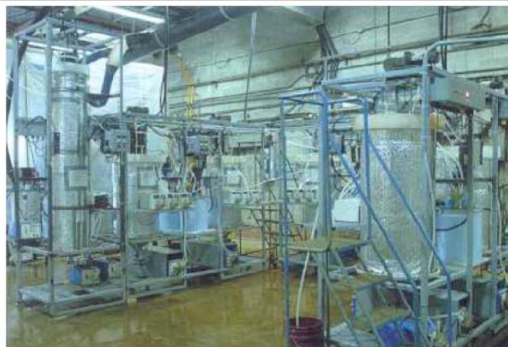
CCD circuit used to do solid liquid separation after pilot-scale leaching.
